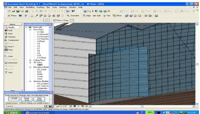
So a change in a window schedule will automatically be carried through to the appropriate plan and elevation,
